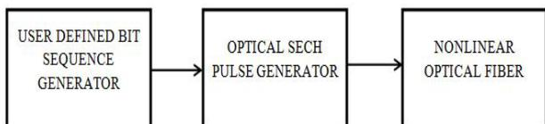
**Figure 4:** Block diagram for generation of Soliton using optical Sech pulse generator
