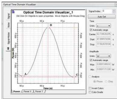
**Figure 14.** One cycle input obtained from pulse after travel 10km
