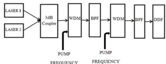
Figure 1: Block diagram for generation of Soliton
