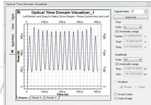
Figure 11: Output Pulse of Gaussian pulse generator after 10km
