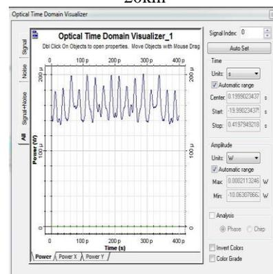
Figure 13: Output Pulse of Gaussian pulse generator after 30km
