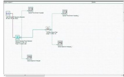
**Figure 5:** Simulation Setup for generation of Soliton using Gaussian Pulse Generator
