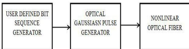
**Figure 3:** Block diagram for generation of Soliton using optical Gaussian pulse generator
