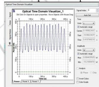
Figure 12: Output Pulse of Gaussian pulse generator after 20km
