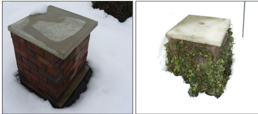
Fig. 4. Snow melt was more rapid around the base of unplanted cuboids (UC) left, compared to planted cuboids (PC) right. Images from 11 Jan 2010 at 15.00 h.
