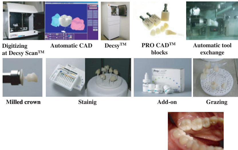
Fig 8. Fabrication of glass ceramic crowns using the CAD/CAM system of Angel crowns™ (Media, Japan).
