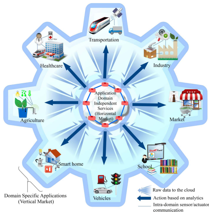
Fig. 1. The overall picture of IoT emphasizing the vertical markets and the horizontal integration between them.
