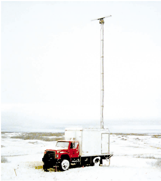
FIGURE 3. Phase Zero radar equipment in Dundurn, Saskatchewan, Canada. X-band clutter surveys were performed at more than one hundred sites.
