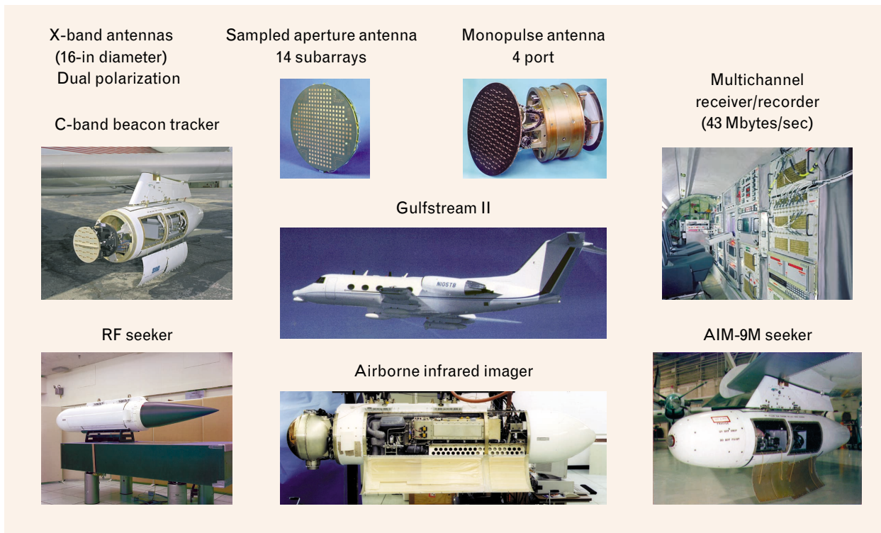
FIGURE 9. Current version of the ASTB. The ASTB is a fully instrumented, highly calibrated, airborne data-collection system. The Gulfstream II platform carries an assortment of sensor pods (e.g., an RF seeker, the airborne infrared imager, and an AIM-9M seeker), a C-band beacon-tracker subsystem that is used to point the sensor pods at beacon-carrying targets, and nose-mounted advanced array antennas. Data from the sensors and support equipment are recorded on a wideband digital recorder for post-mission data analysis and interpretation.
