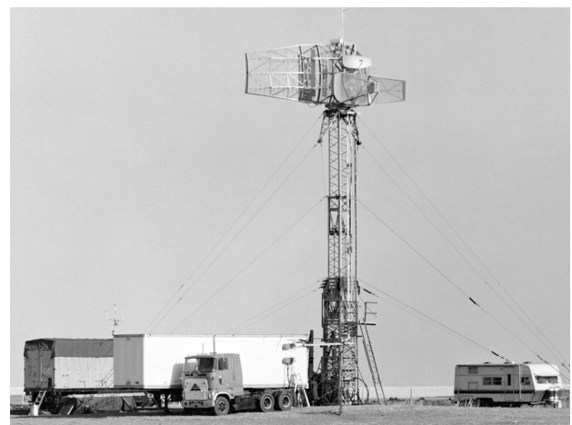
FIGURE 4. Phase One radar equipment at Lethbridge, Alberta, Canada. Clutter surveys at five different frequencies were performed at forty-two different sites.
