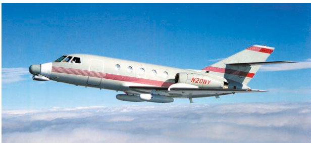
FIGURE 7. Dassault Falcon-20 twin-engine jet aircraft. This platform was the original Airborne Seeker Test Bed (ASTB).
