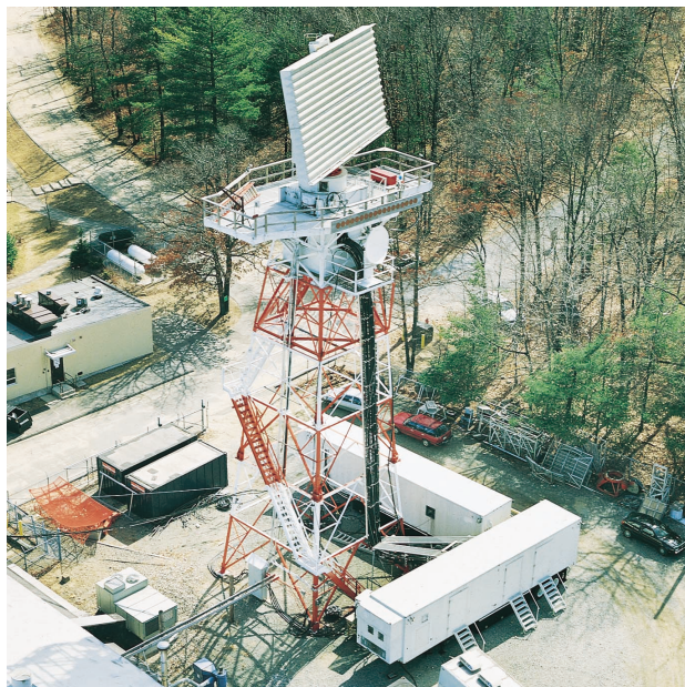
FIGURE 10. Radar Surveillance Technology Experimental Radar (RSTER), as originally deployed at Lincoln Laboratory. The 5-m-high \times 10-m-wide, 14-channel antenna is connected to the transmitter and receiver subsystems via a 33-channel rotary coupler. Signals from the individual channels are digitized and processed to achieve adaptive digital beamforming (in elevation), pulse compression, Doppler filtering, constant false-alarm-rate detection, multitarget tracking, synthetic displays, data recording, and target track-file generation. The last capability is required to direct other sensors and weapon systems. All the radar subsystems are contained in the two forty-foot trailers shown at the base of the tower.
