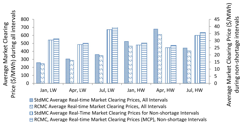
Fig. 4. Average real time market-clearing prices overall and in non-shortage intervals. The RCMC algorithm tends to have slightly higher prices in non-shortage intervals, but much lower prices overall, as shortages (and the associated high prices) are reduced relative to the StdMC algorithm.
