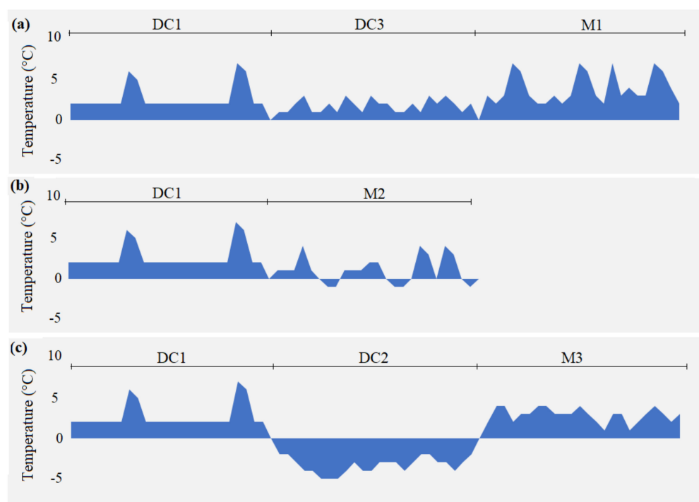
Figure 2. Temperature profile based on hourly variation during a 1-day period to represent distribution centers (DC1, DC2, and DC3) and markets (M1, M2, and M3) in logistic distribution routes R1 (a), R2 (b), and R3 (c). DC2 was eliminated from R1 due to insignificance of microbial growth once products were stored at a temperature profile constantly below zero, keeping frozen storage temperatures.
