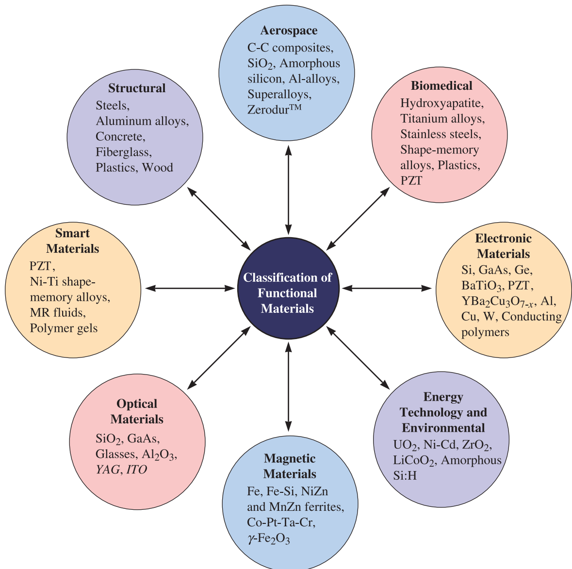
Figure 1-6 Functional classification of materials. Notice that metals, plastics, and ceramics occur in different categories. A limited number of examples in each category are provided.
