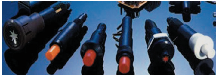
Figure 2-2 Piezoelectric PZT-based gas igniters. When the piezoelectric material is stressed (by applying a pressure), a voltage develops and a spark is created between the electrodes. (Courtesy of Morgan Electro Ceramics, Ltd., UK.)
