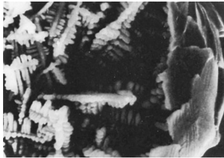
Figure 9-26 Dendrites in a titanium powder particle produced by rapid solidification processing ( \times 2200 ) (for Problem 9-43). (From J.D. Ayers and K. Moore, "Formation of Metal Carbide Powder by Spark Machining of Reactive Metals," in Metallurgical Transactions, Vol. 15A, June 1984, p. 1120.)
