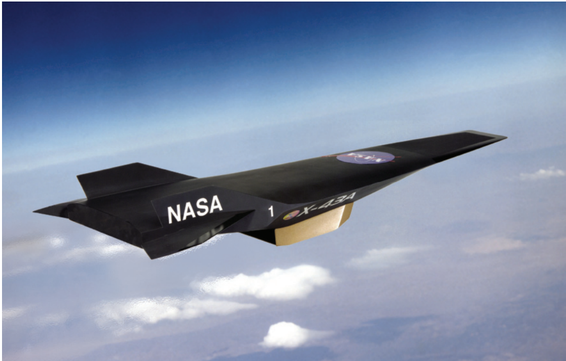
Figure 1-9 NASA's X-43A unmanned aircraft is an example of an advanced hypersonic vehicle. (Courtesy of NASA Dryden Flight Research Center (NASA-DFRC).)
